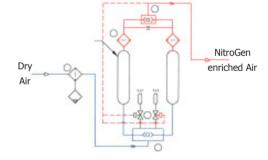
The Typical installation is for On-site Gas Generation as per below.
