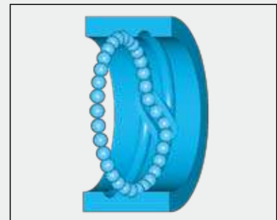
Fig 3.5 Circuit for internal return cap
